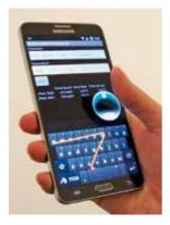
SWiM - or Shape Writing in Motion interprets the wrist motion of the dominant hand to trace an input. The tilting motion controls a pointer ball, which traces a path for the gesture keyboard with one word resulting from each gesture.
